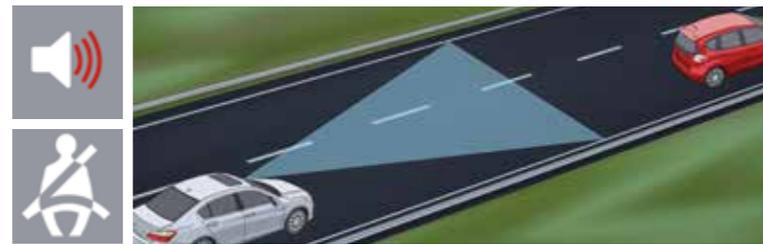
Primary warning: When there's a risk of collision ahead, or the distance between the two vehicles is too short, the alarm sounds and the word BRAKE appears on the i-MID (Intelligent-Multi Information Display). This alerts the driver to take action in order to avoid collision.
